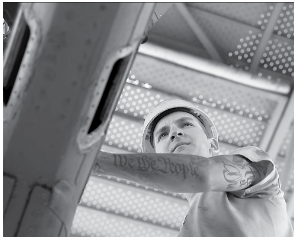
Senior Airman Andrew Dashler, 60th Maintenance Squadron KC-10 Extender inspection technician, checks the tension cable on the boom of a KC-10 Extender July 23 at Travis Air Force Base, Calif. The inspection crew was performing 1A inspections where they depanel, lubricate, check flight controls and follow through with in-depth inspections of all major areas, which include the aircraft tail, boom, wings and gear components.
